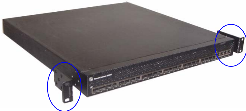
Figure 1. Attaching the Brackets
