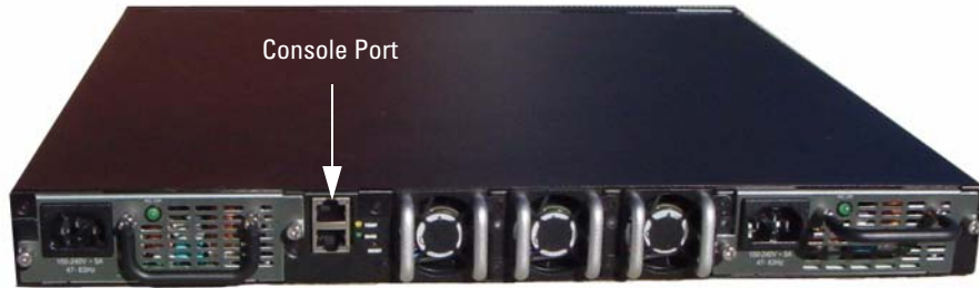
Figure 3. Connecting to the Console Port
