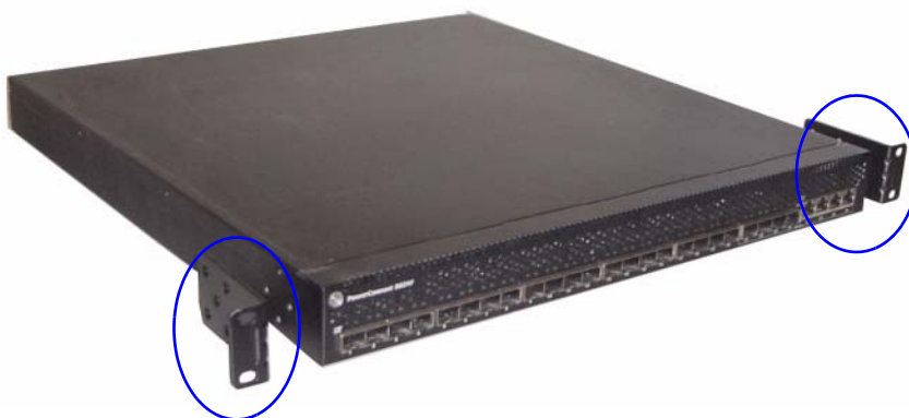
Figure 1. Fixation des supports
